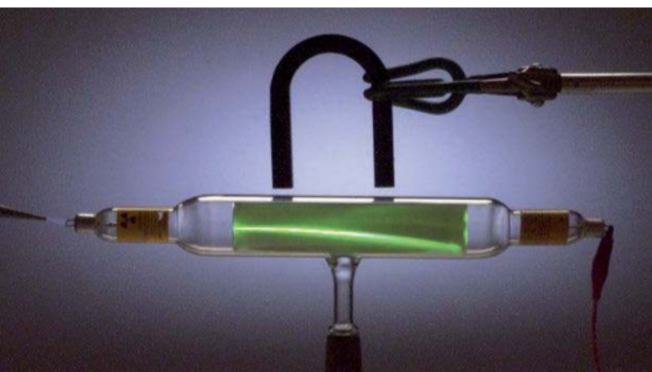
■ Figure 2.8 Cathode rays are streams of electrons, produced in a glass tube like this containing a vacuum, from charged metal electrodes. Cathode rays are invisible, but they cause a phosphorescent screen to glow so we can see their path. They are deflected by a magnet, which tells us that they are electrically charged.
